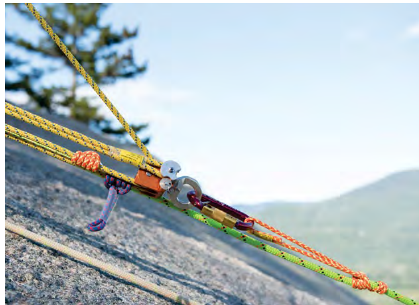
(Upper) AZTEK with SuperStatic2™ and SafeD carabiners as part of a rescue litter system. (Lower) AZTEK with WorkPro™ as part of a piggyback haul setup.
