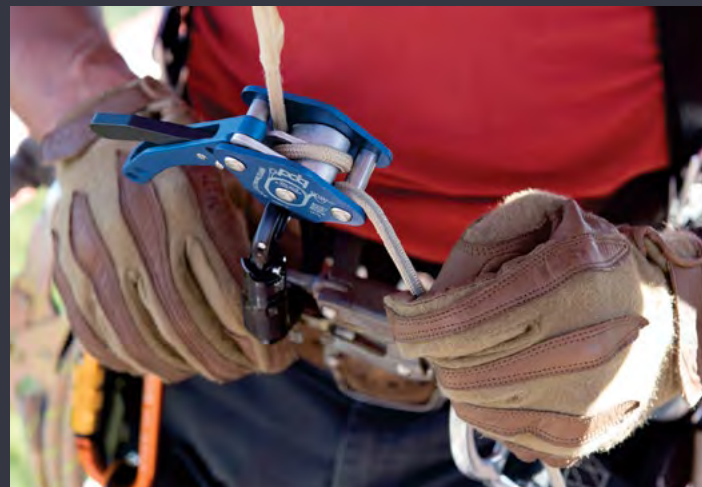
(Clockwise from top) Tower worker descending with PDQ System. PDQ set up as progress capture in pick off raising system. PDQ device in autolock mode.
