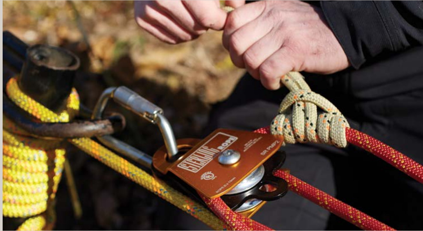
9 mm RIT Bound Loop Prusik used for progress capture in the Tree Pulling Kit (see pg. 19).
